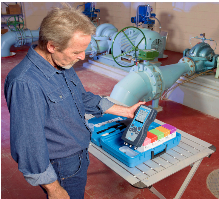
Hach SL1000 and all the operator's required testing parameters included in a single carrying case.
