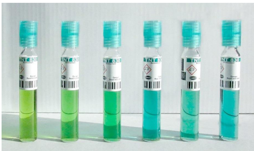
Figure 1: Cuvettes 1–3 within the measurement range, cuvettes 4–6 with too high ammonia nitrogen content
