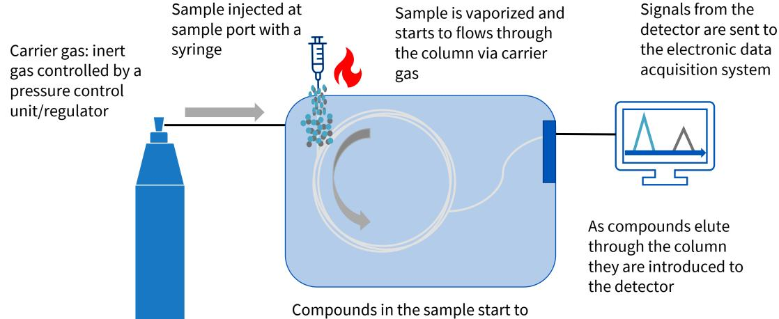
CTE GLOBAL, INC. Leading to a brighter tomorrow Compounds in the sample start t separate in order of boiling point/polarity
