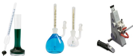
Figure 1: Conventional setups to measure °Brix. From left to right: hydrometer, pycnometer, Abbe refractometer.
